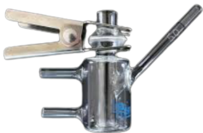
Figure 5: Franz Cell used to measure the penetration of free \alpha -arbutin and SalSphere® Light containing \alpha -arbutin at the same dosage.
