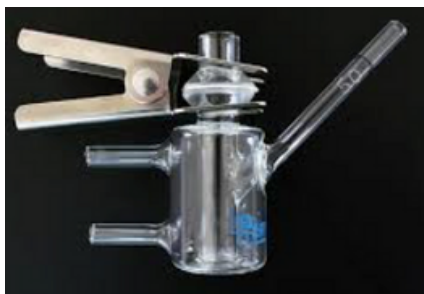
Fig 3: Franz Cell used to measure the penetration of free \alpha -arbutin and SalSphere® Light containing \alpha -arbutin at the same dosage.
